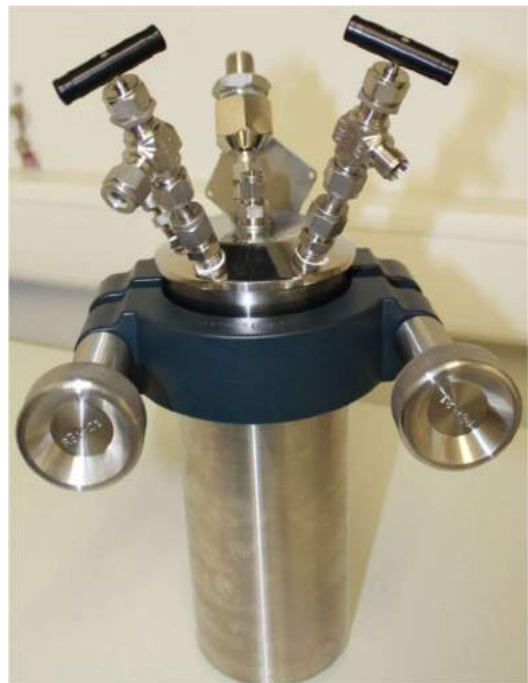
Figure 2: CO 2 high-pressure autoclave, in the picture a version without temperature and pressure sensor
