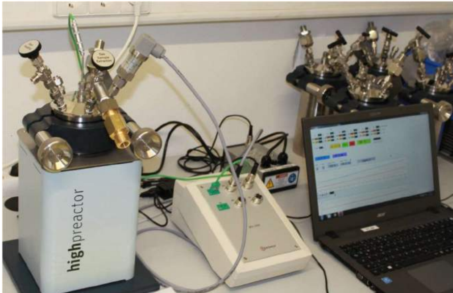
Figure 2: Workplace with CO 2 high-pressure autoclave with pressure and temperature sensors for continuous recording of these parameters. The autoclave is located in a controlled heating block.
