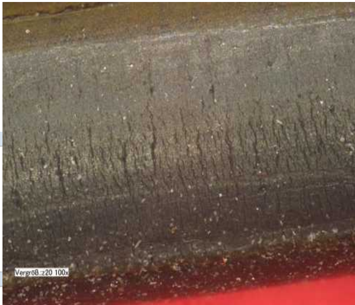
Figure 8: Cracks on the contact surface of an O-ring due to aging through heat and oxygen, made visible through slightly stretched condition
