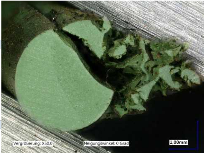
Figure 6: Strong swelling which resulted in shear
