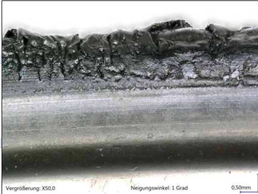
Figure 3: Chemical degradation and swelling with blistering
