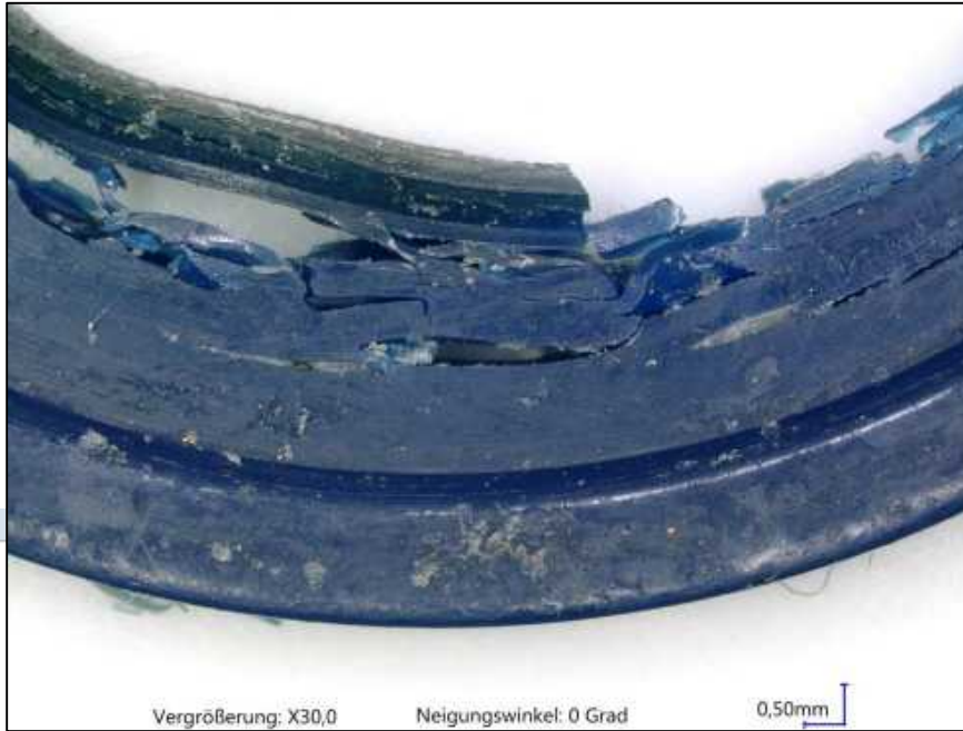
Figure 4: Hydrolysis (= chemical degradation by water) of a poly-urethane seal
