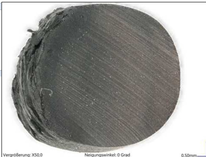
Figure 2: Chemical degradation on FKM-material by an inorganic acid
