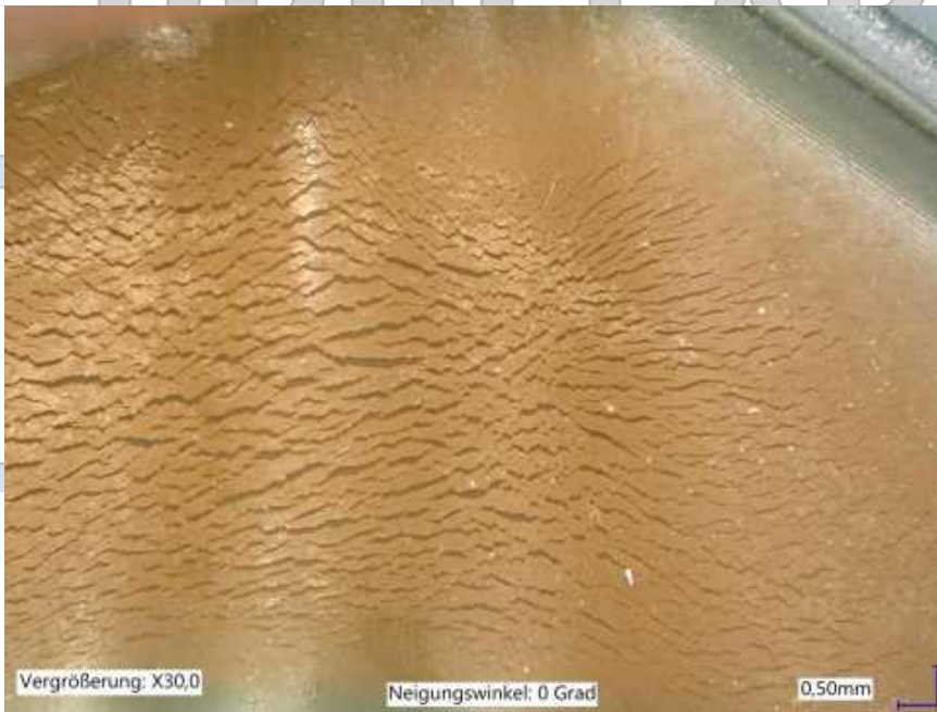
Figure 5: Chemical degradation on FVMQ-membrane probably by blow-by-gas in engine oil
