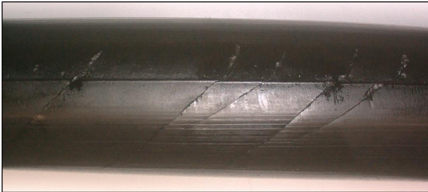
Figure 2: Example 1 - Cracks on the outer diameter
