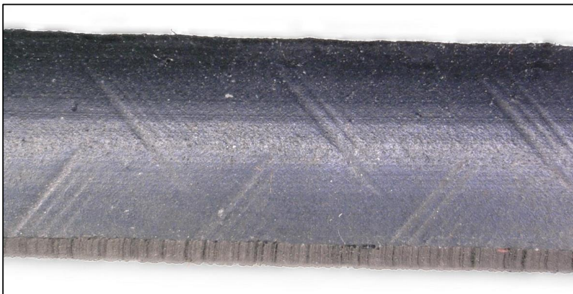
Figure 10: Example 3 - New material (new supplier) after ozone test
