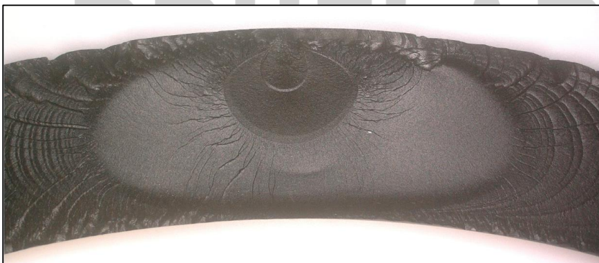
Figure 3: Example 1 - Fracture surface
