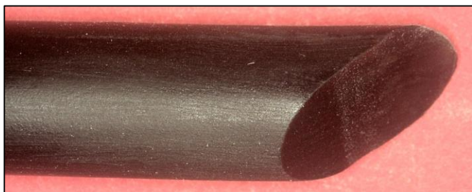
Figure 4: Example 2 - Torn joint
