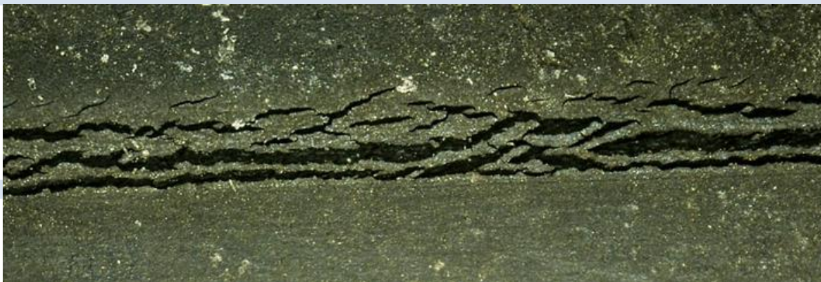
Figure 3: Cracks on a static pre-stretched bellow made of a BR/IR-elastomer
