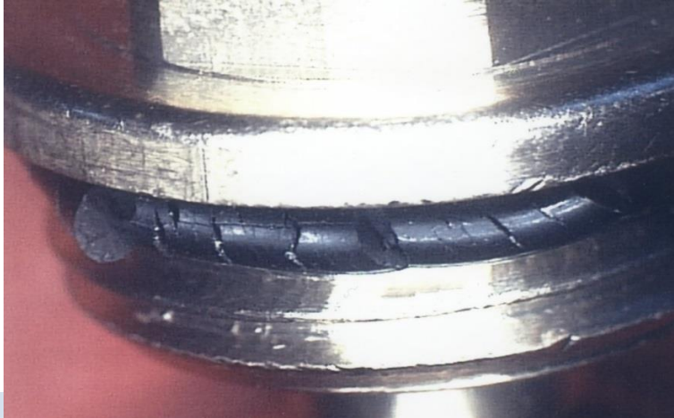
Figure 1: Pre-installed NBR O-Ring, severely cracked after several weeks of storage
