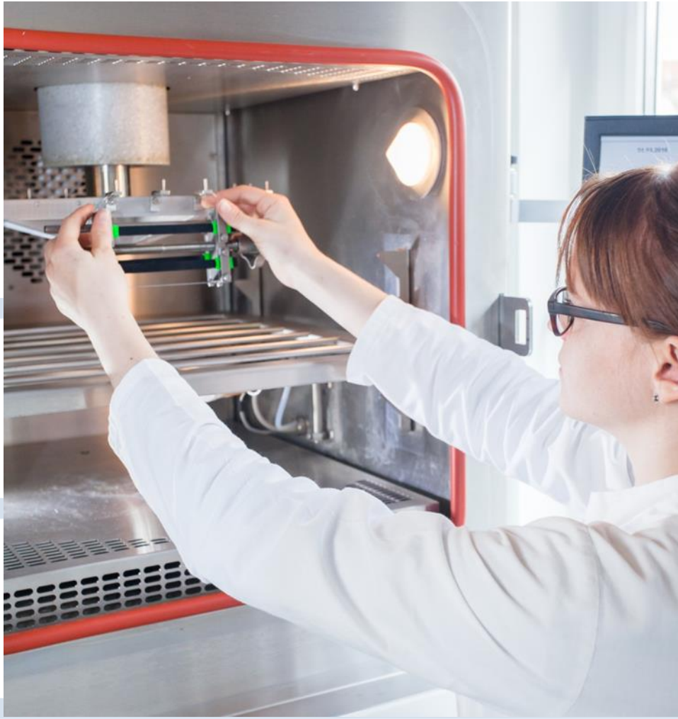
Figure 7: Performance of ozone test: Employee of Richter O-Ring Test Laboratory in front of an open ozone cabinet
