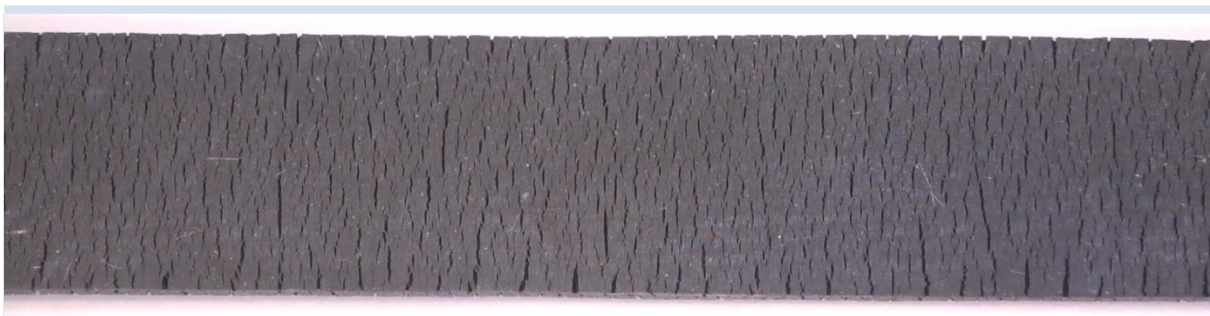
Figure 6: Example of elastomer specimen after ozone test (condition after 48h / 40°C / 20% stretching / 50 pphm ozone concentration / 55% relative humidity): Sample is still in stretched condition and has long, moderately wide cracks (stage 2 assessed based on DIN 53509) (10x magnification)
