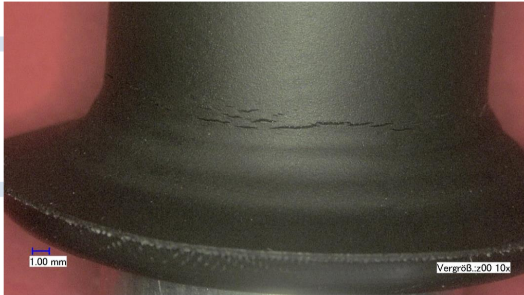
Figure 4: Fatigue cracking on FKM-membrane
