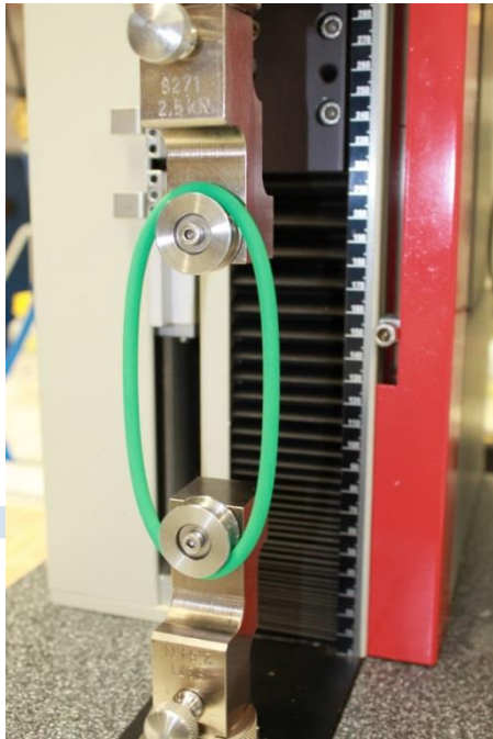
Fig. 8: Tensile test of an O-ring on ball bearing rollers (here not driven)
