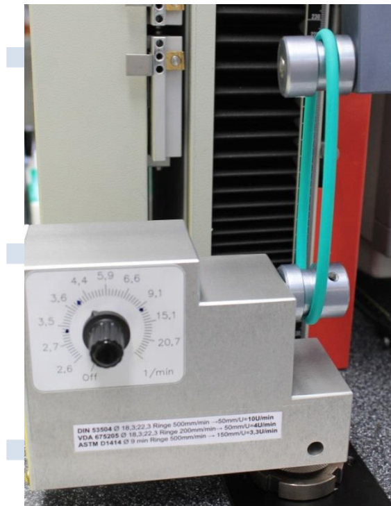
Fig. 6: Tensile test with driven roller: The drive unit can be seen at the bottom left of the picture. The rotation speed of the roller is variably adjustable, depending on the requirements of the corresponding standard.
