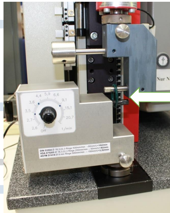
Fig. 7: Tensile test of a small dark green O-ring with a driven roller and a smaller diameter.
