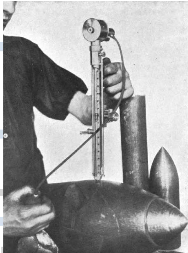
Fig. 2: A Shore scleroscope with a vertical scale from 1910 shown in a book by Albert F. Shore regarding his scleroscope. 6 A worker determines the hardness of a bullet.
