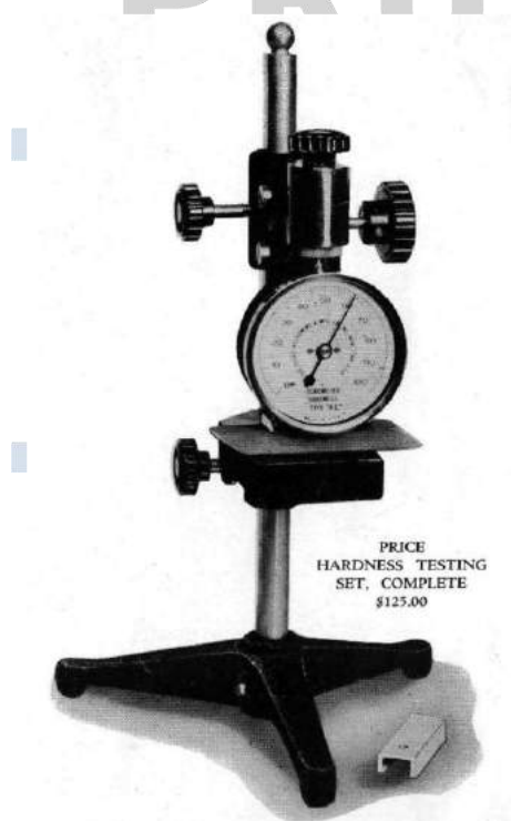
Fig. 10: Presentation of the round Shore A measuring instrument of Shore Instrument &MFG Co., Jamaica, N.Y. with stand (introduced 1944). It received the designation "A2-Durometer". 42 With the rotary knob on the right above the durometer, it could be moved up or down. At the beginning of the 1950s, a stand from ZWICK & Co KG was already available, which pressed the durometer against the sample
