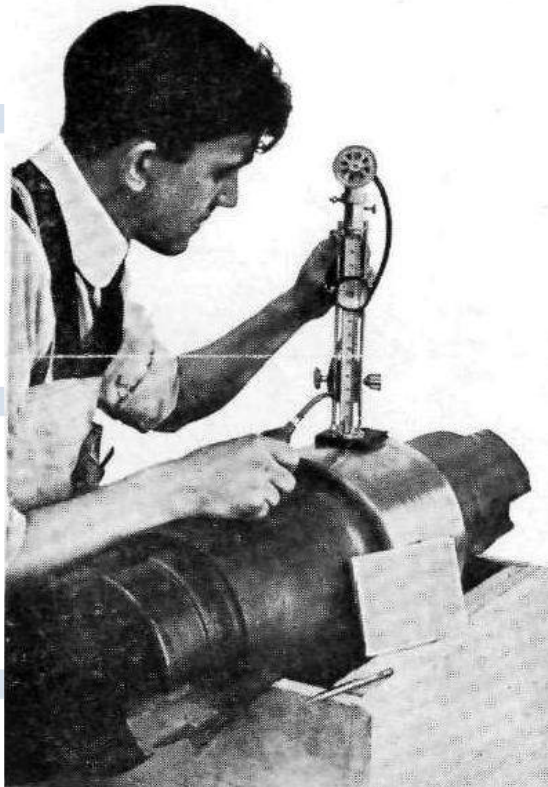
Fig. 1: Presentation of a Shore scleroscope with a vertical scale from an early company brochure of "The Shore Instrument & Mfg. Co. Inc." 5 A worker determines the hardness of a metal shaft.
