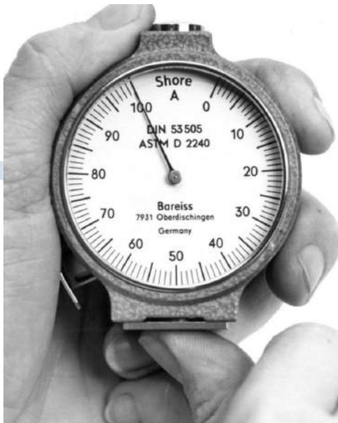
Fig. 17: A historical round pocket tester HP from Bareiss, already with a division of the degrees of hardness into single steps (Photo: Bareiss Prüfgerätebau GmbH, www.bareiss.de)
