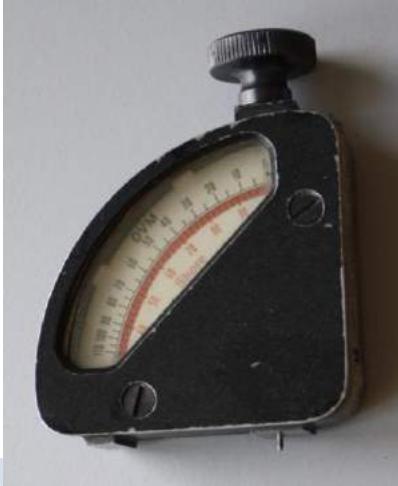
Fig. 29: From early on, attempts were made to convert ShA hardness grades into other hardness units. The historical durometer (classic "quadrant type") from Zwick shown on the left is an interesting example of a double scale with ShA hardness (red scale) and DVM softness number (black scale). 100 (Photo: Zwick GmbH & Co. KG, Ulm)
