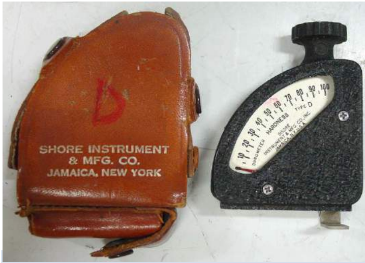
Fig. 11: A later example of a Shore D handheld tester ("quadrant type") with leather case, (permission to reproduce courtesy of "Toronto Surplus & Scientific", Canada)
