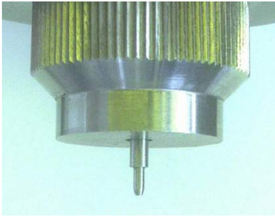
Fig. 26: Indenter and pressure surface of a Shore A test unit (magnification fivefold) (Photo: G. Reiner, O-Ring Prüflabor Richter GmbH)
