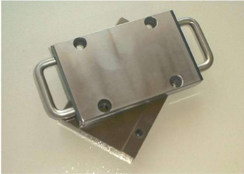
Figure 6: The O-Ring Prüflabor Richter GmbH owns numerous sets of tools for testing of compression set with base plates ground to different depths (see the lower plate in the picture), so that the insertion of spacers can be dropped)
