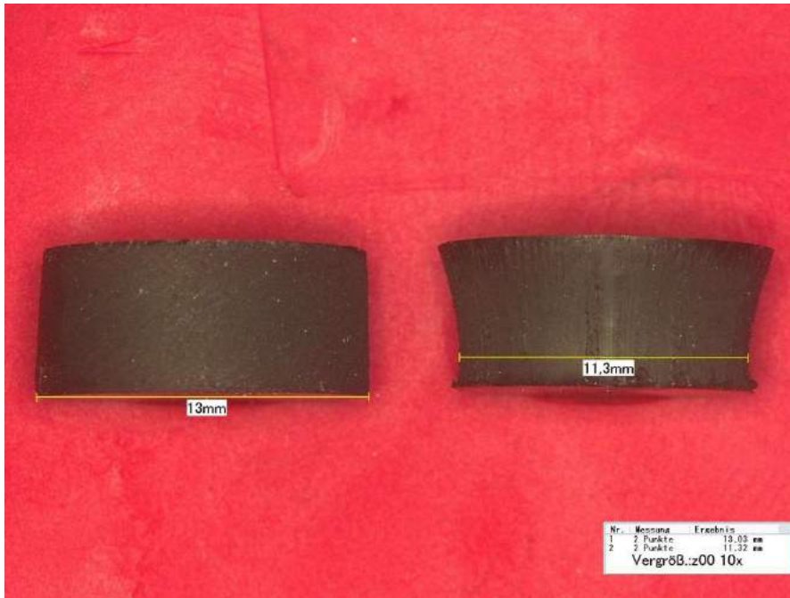
Figure 9: The die-cut test piece can be identified on the right side, the one, cut out by a rotary knife, is on the left. In the case on hand the smallest diameter of the die cut test piece (11,3mm) differs up to 13% from the specified size (13mm)! (Magnification 10x).
