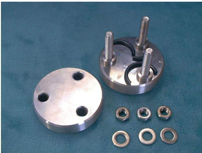
Figure 7: Flat plates for compression set measurement with spacers. Compression set tools as used at the Prüflabor Richter for compression set testing in media. Their round shape allows their deposition into a glass beaker without problems.
