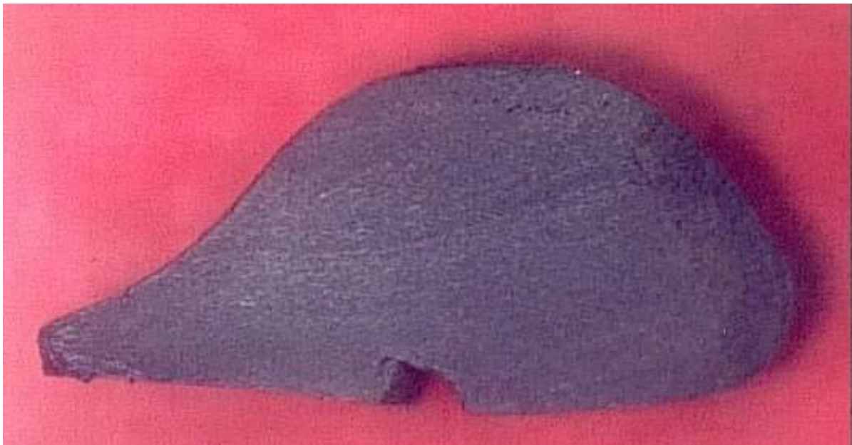
Figure 4: FKM O-ring after several weeks of use at 175°C in a press fitting and 175°C water temperature
