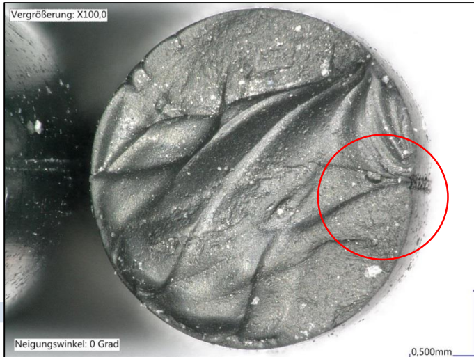
Fig. 10: Ruptured O-ring due to vulcanization defect: Inhomogeneous and fissured fracture surface
