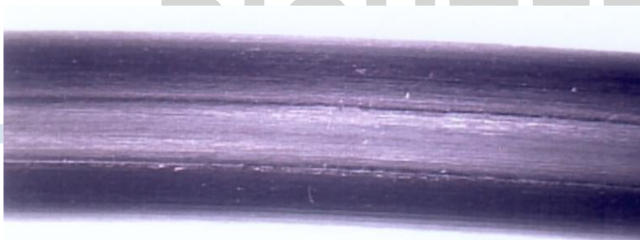
Fig. 8: Crack caused by a sharp edge during assembly
