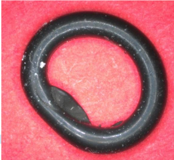
Fig. 2: Crushing due to incorrect positioning of the seal
