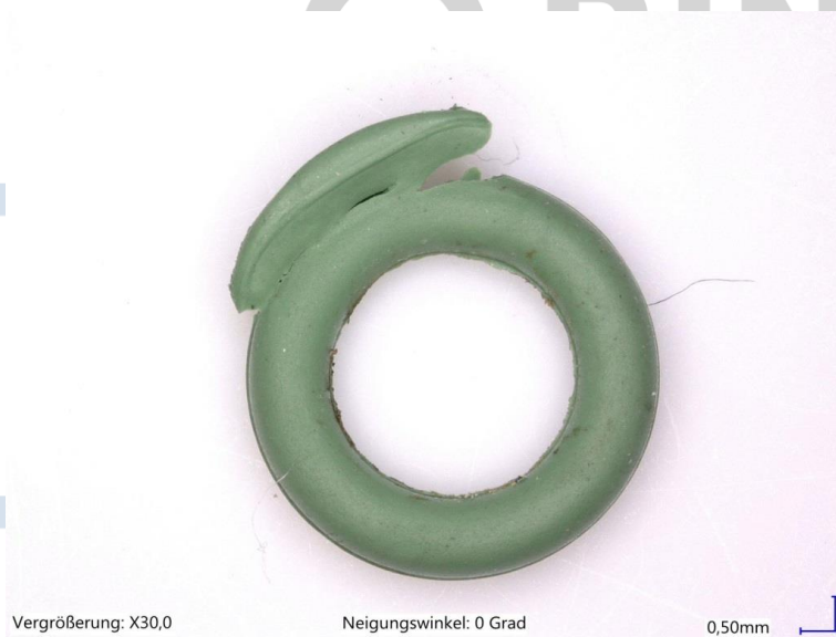
Fig. 3: O-ring with crushed area during assembly
