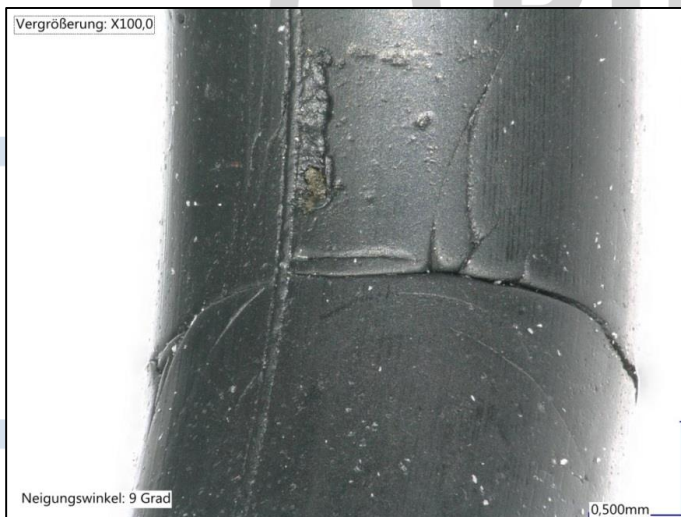
Fig. 11: Vulcanization defects due to manufacturing: Rounded crack transition
