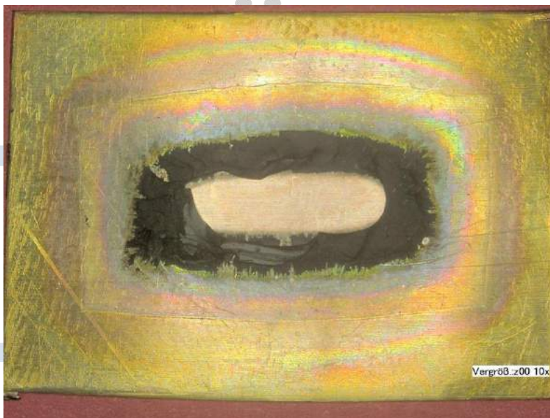
Fig. 9: Remains of a large-area bonding of a test specimen to a copper plate: Such an elastomer is considered susceptible to autoxidation.
