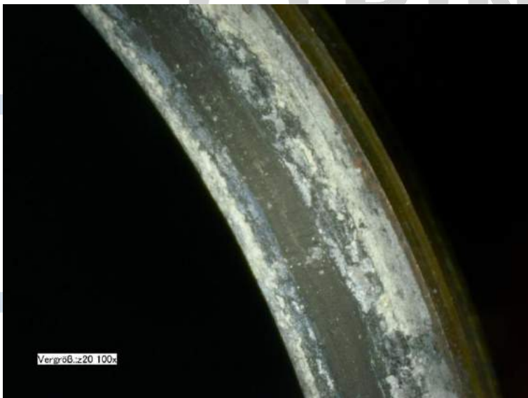
Fig. 7: Opposite surface of the EPDM O-ring from Fig. 6, the white areas are probably lime deposits.
