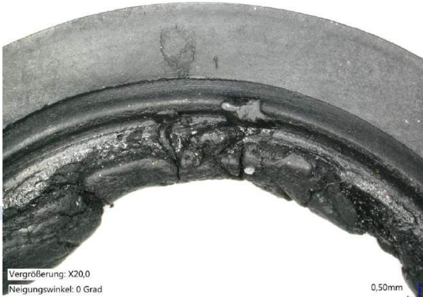
Fig. 4: An elastomer damaged by autoxidation (peroxidically cross-linked EPDM), which has clearly fused areas in the interior of the sealing ring, similar to a thermoplastic or TPE.
