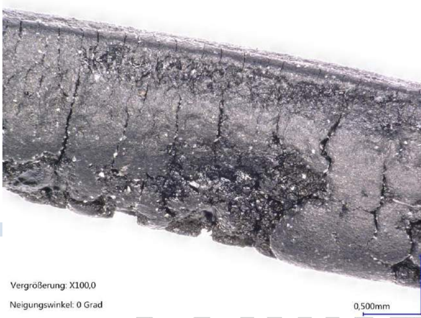
Fig. 2: EPDM O-ring, peroxidically cross-linked after use in a monitored endurance test for a water fitting (cause of damage: dezincification of brass, cyclic temperature changes from 25°C to 95°C in water, test duration 4500 h)
