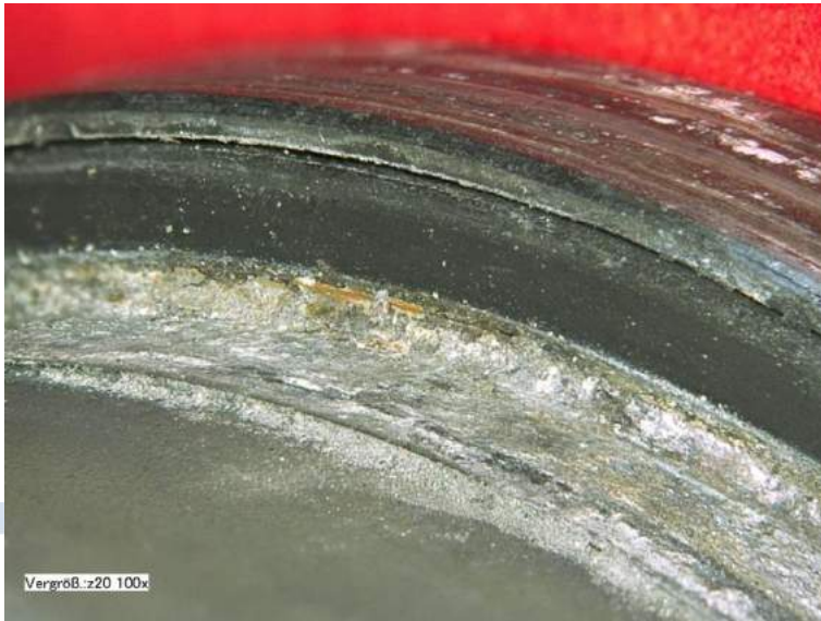
Fig. 6: EPDM O-ring after autoxidation in the installed state, permanently deformed and with a sooty surface
