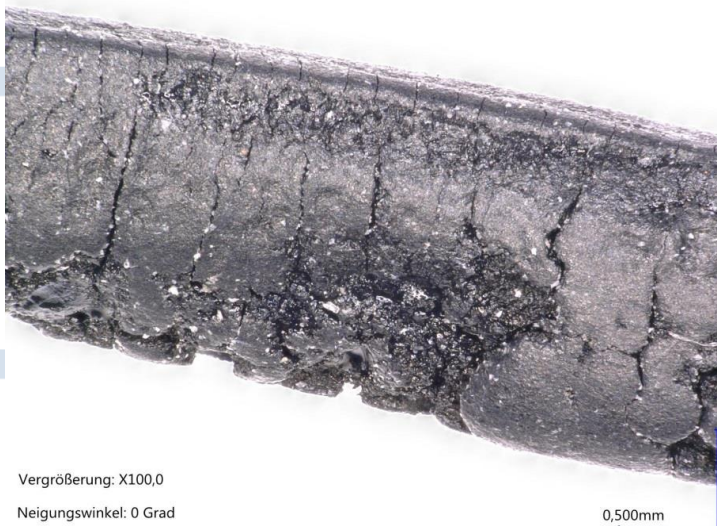
Fig. 1: EPDM O-ring, perox. cross-linked after endurance test (cyclic temperature change from 25 to 95° C in water with Cu ions, test duration 4500 h)
