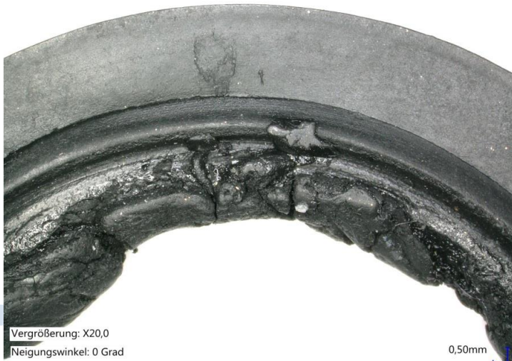
Fig. 2: EPDM seal damaged by autoxidation (dezincification) with clearly visible fused areas, similar to a thermoplastic or TPE
