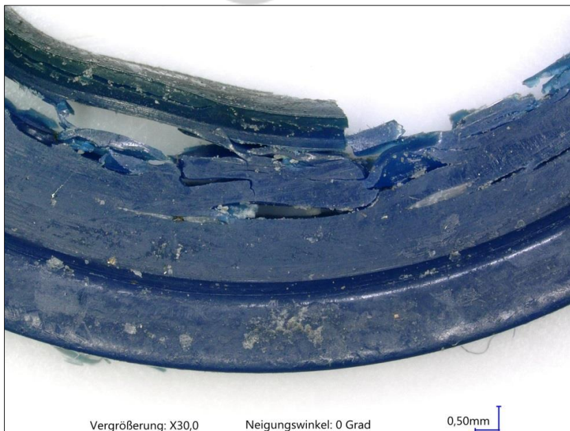
Fig. 3: Hydrolysis (= chemical erosion by water) of a polyurethane seal
