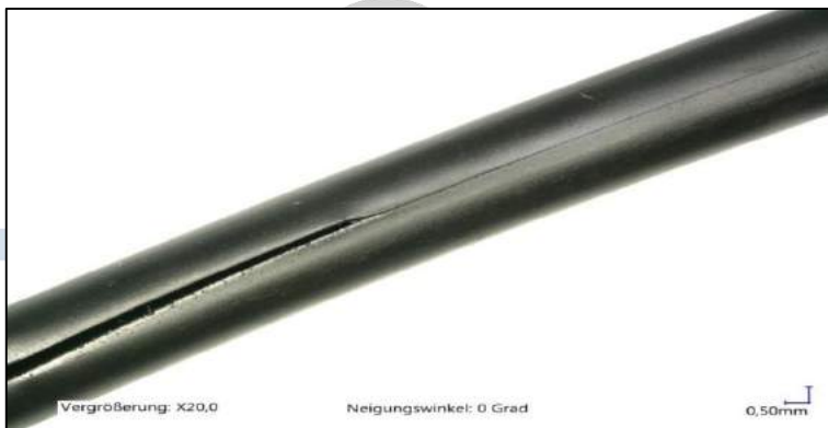
Fig. 24: Installation crack due to the impact of a sharp edge in the installation space
