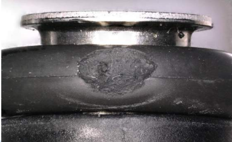
Fig. 23: Chipping out during assembly: The damage occurred at room temperature and resulted in a non-smooth fracture surface; the characteristics of the fracture surface are also strongly dependent on the tear resistance of a material.
