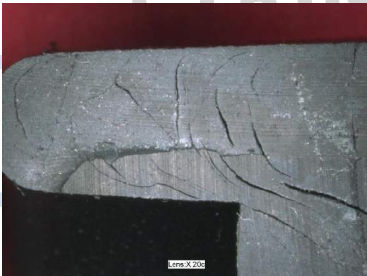
Fig. 8: Production-related cracks due to a superimposed compound
