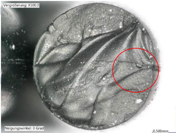
Fig. 6: Torn O-ring due to vulcanization defect: Inhomogeneous, fissured fracture surface
