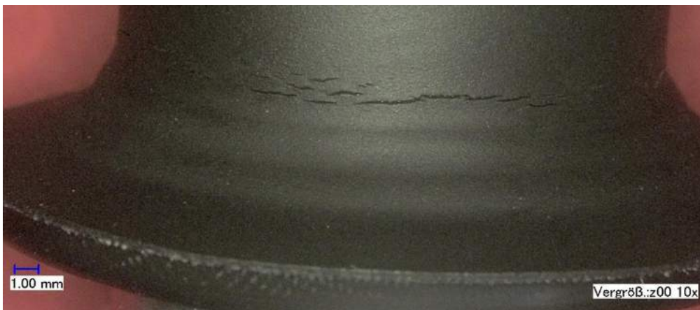
Fig. 20: Fatigue cracks on an FKM membrane
