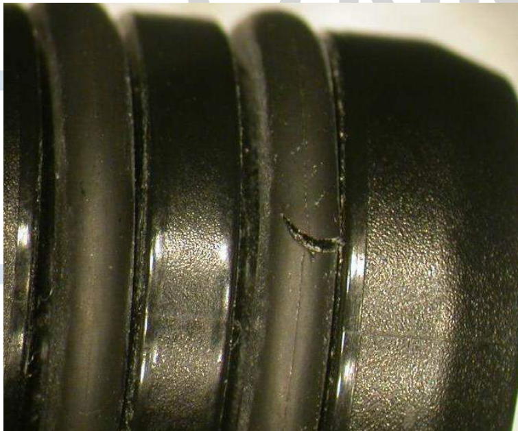
Fig. 2: Crack due to a vulcanization defect, recognizable by the parabolic crack shape symmetrical to the mold parting line
