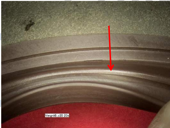
Fig. 15: Demolding crack on a molded gasket
