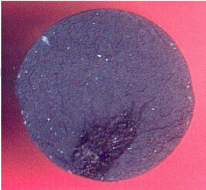
Fig. 11: Crack triggered by foreign material entry
