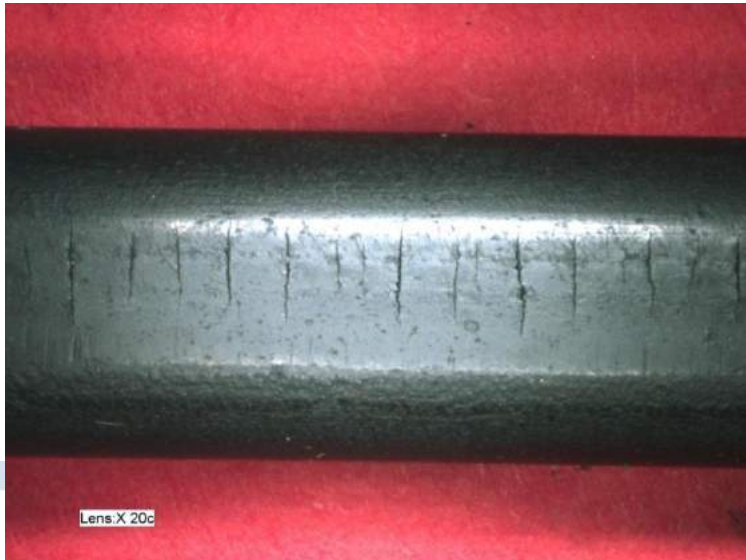
Fig. 21: Thermally damaged O-ring, fully hardened, cracks visible on the contact surfaces when bending
