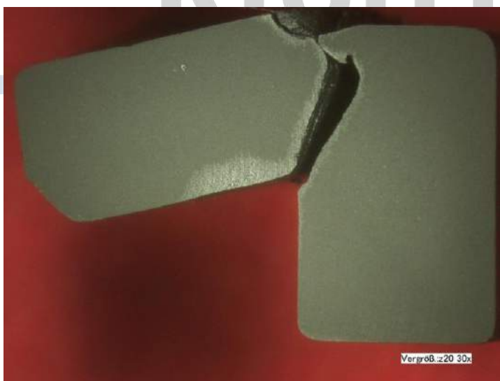
Fig. 16: Demolding crack at a sealing element
