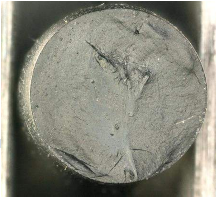
Fig. 5: Torn O-ring caused by a vulcanization error
