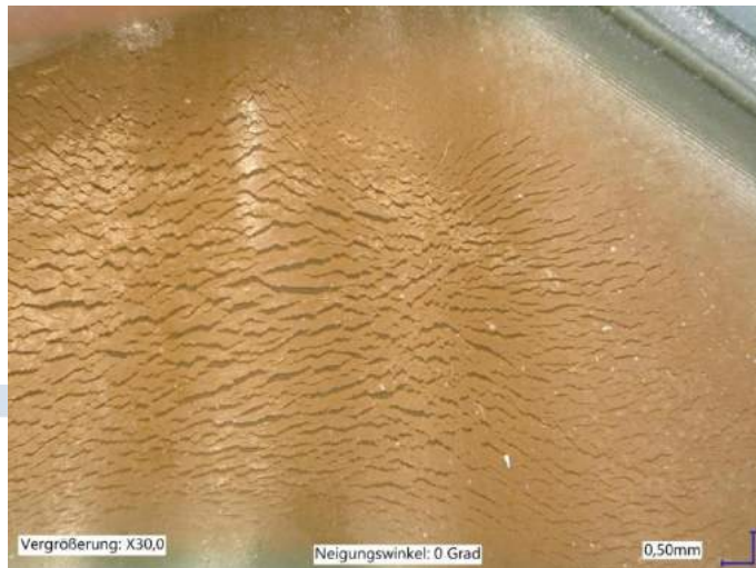
Fig. 26: Chemical degradation of an FVMQ membrane: The cracks cover a larger area.
