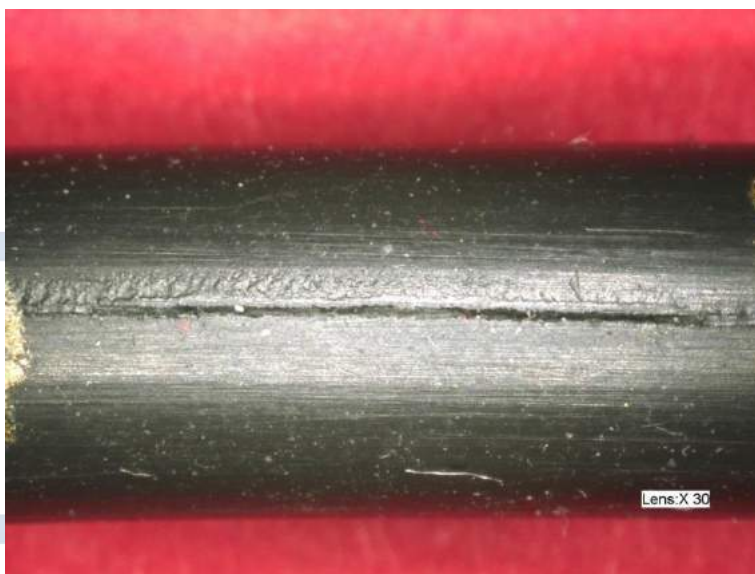
Fig. 12: Shrinkage crack on an O-ring
