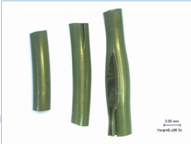
Fig. 1: Cracks in an FKM O-ring due to over-vulcanization after a compression set test of 168h / 200°C
