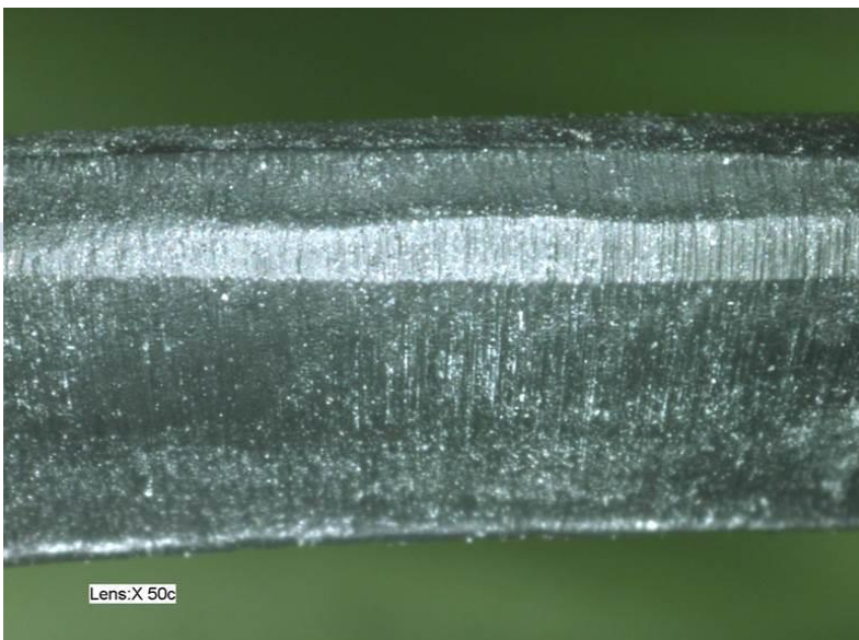
Fig. 10: Top view outside diameter of the damaged O-ring from Fig. 7
