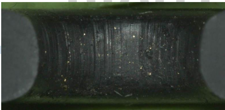
Fig. 4: Inside of a cut EPDM O-ring from a thermostatic valve: Metal particles are clearly visible in the grooves (hydroabrasion).
