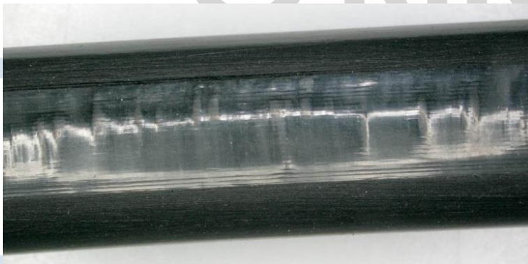
Fig. 3: Unsymmetrically flattened O-ring, the abraded surface is smooth and shiny.
