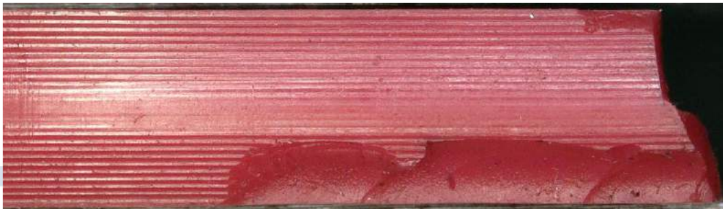
Fig. 13: Damage to a thermoplastic polyurethane seal at the sealing gap after strong chemical impact and resulting loss of strength.
