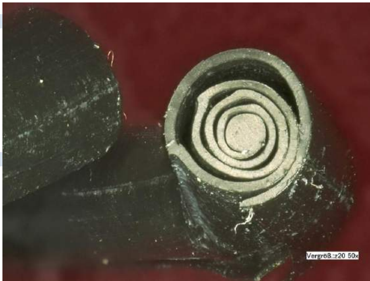
Fig. 5: Damage pattern of a gap extrusion, formed at 350 bar pressure and a gap of 0.05 mm, atypically and strongly formed as a result of a sharp-edged groove recess.
