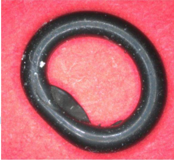
Fig. 16: Damage caused by a mounting error (compression)
