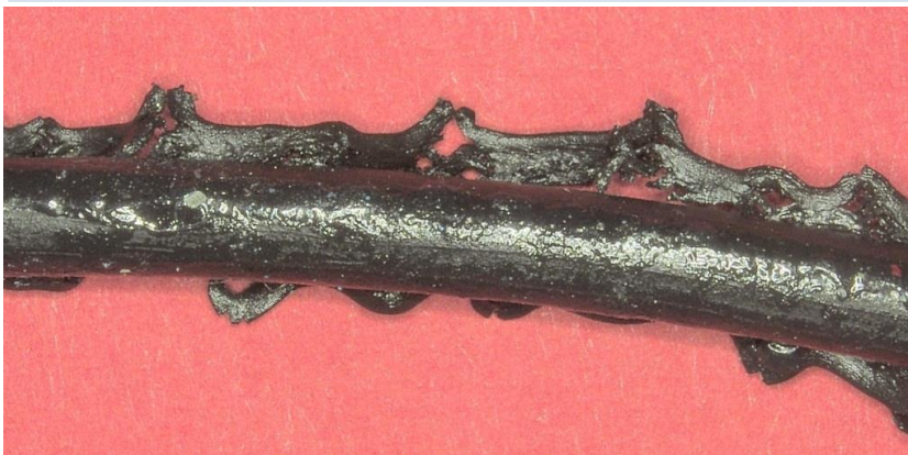
Fig. 2: O-ring cross-section after a typical groove overfill: The crushed areas can be seen above and below
