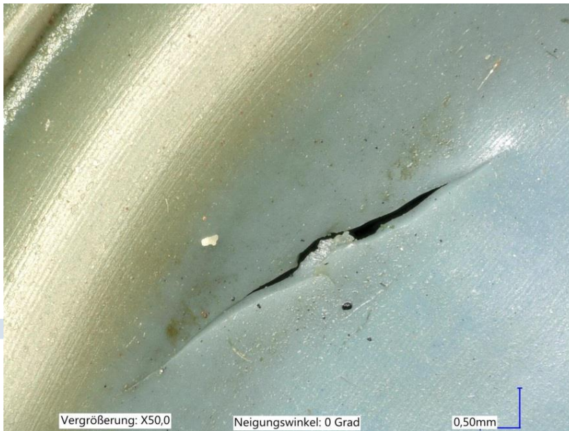
Fig. 5: Incision on a membrane through a sharp edge in the installation space.
