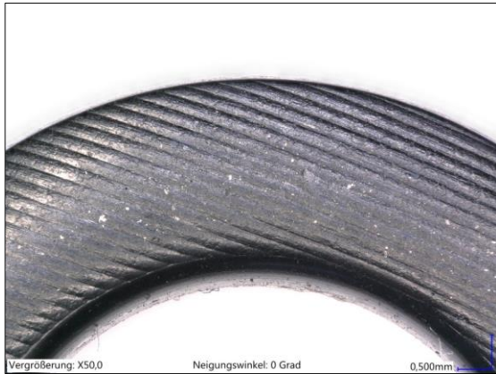
Fig. 7: This reason for failure due to an unsuitable surface structure of the groove can be clearly seen under the microscope, as the poor surface is visibly imprinted on the elastomer: The leakage is caused by the deep scoring in the groove.
