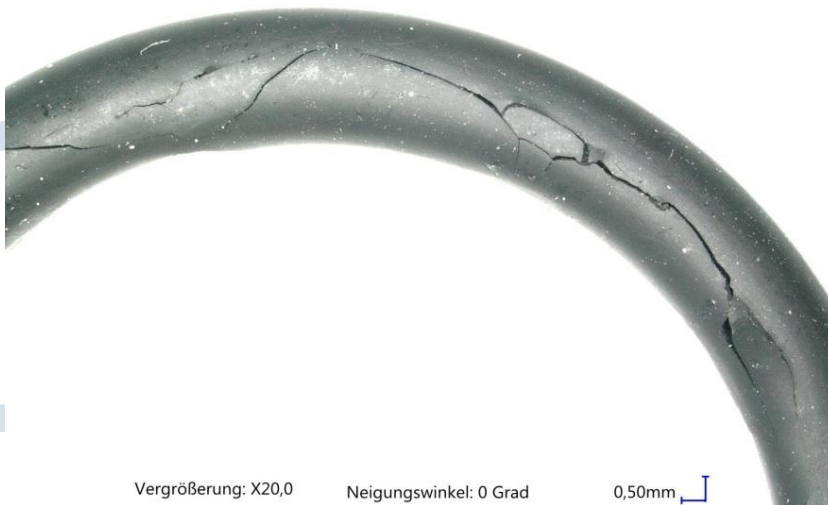
Fig. 4: EPDM O-ring, destroyed by excessive deformation and thermal impact (stress cracks)
