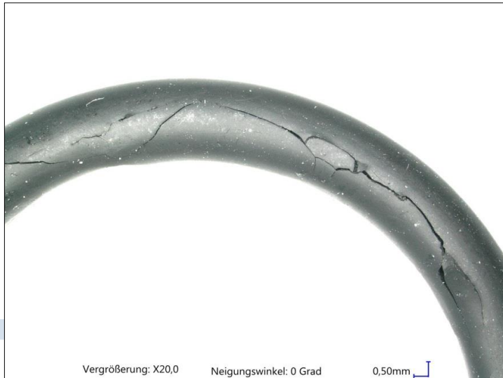
Fig. 3: EPDM O-ring, destroyed by excessive deformation and thermal impact (stress cracks)
