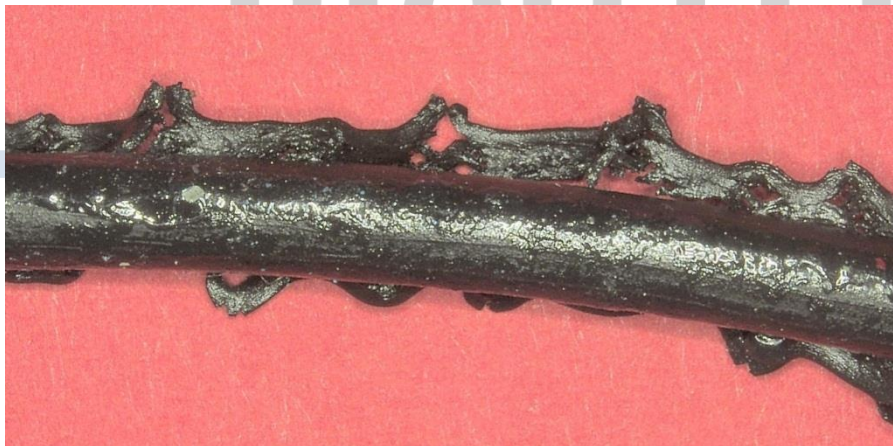
Fig. 2: O-ring cross-section after a typical groove overfill: The squeezed areas can be seen above and below.
