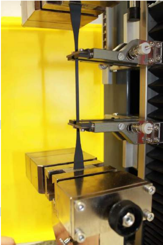
Fig. 6: Stretched dumbbell rod, shortly before tearing. The extensometers now rest against the dumbbell rod and measure its elongation in the standardized measuring range. Here you can see how the cross-section of the measuring range narrows due to the elongation.
