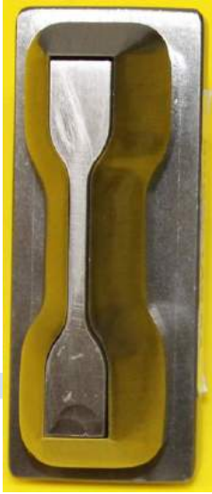
Fig.9: Typical punching tool: The tool has a spring activated ejector for the dumbbell rods.
