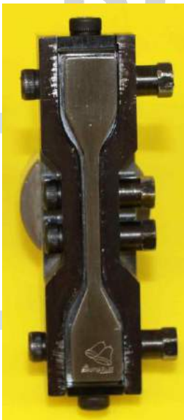
Fig. 10: Punching knife: The screws on the punching knife are necessary for changing the blades. The tool also has a spring activated ejector for the dumbbell rods.
