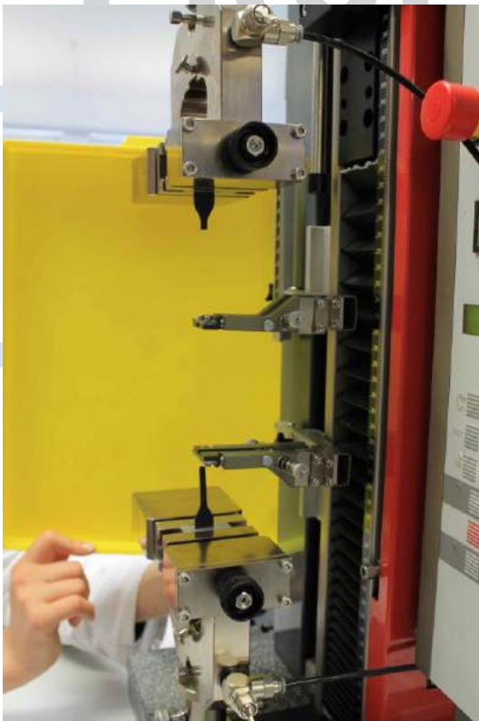
Fig.7: The torn dumbbell rod is removed from the clamping jaws. This is the end of the tensile test.
